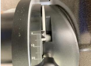
A close-up view of the DOB10's base showing the angle adjustment mechanism. A scale is visible, ranging from 0 to 20 degrees.                                           | DOB10 の水平アングルを 0 度に合わせる。                                                                          |
