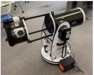
The final setup of the DOB10 telescope, showing the telescope mounted on the base, which is now level and pointed towards true north.                                 | この時点でこんな感じになるはず。<br><br>水平・真北に設置されているか確認。                                                         |
